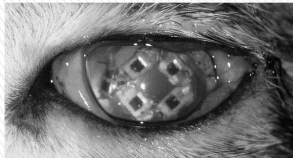
Epi-retinal electrical stimulator powered by an array of PIN diodes [2]
